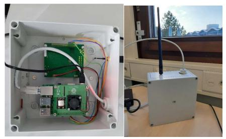
Figure 2: Prototype of LoRaWAN Gateway
