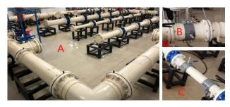
Figure 1. Full-scale water distribution system experimental device
