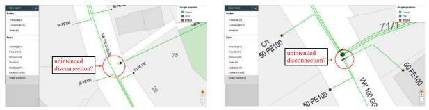
Figure 8: Possible sources of disconnection: distant node (left), valve closure (right)
