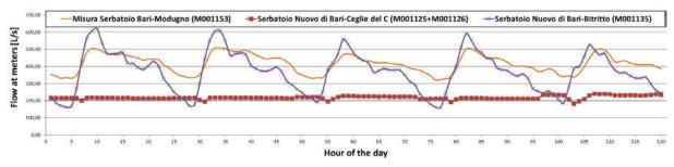
Figure 7. Hourly average flow rate measured at the three reservoir of Bari City subnet.
