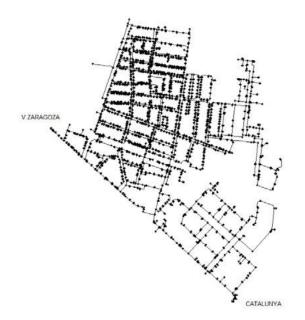
Figure 2. Hydraulic model of Benimaclet sector in Epanet [Source: ]
