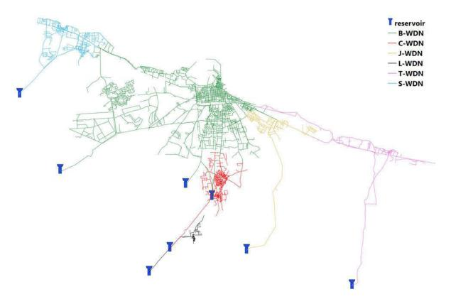
Figure 1. Visualization of the real WDN layout and its sub-networks.
