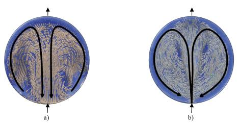
Figure 8. CFD results at mid water height for circular tanks: a) plunging jet and b) submerged jet.
