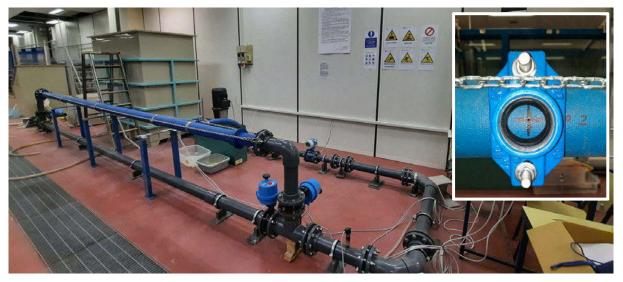
Figure 3. View of the hydraulic system after modifications; particular of the cast-iron pipe with hole used in the experiments (box on the right)
