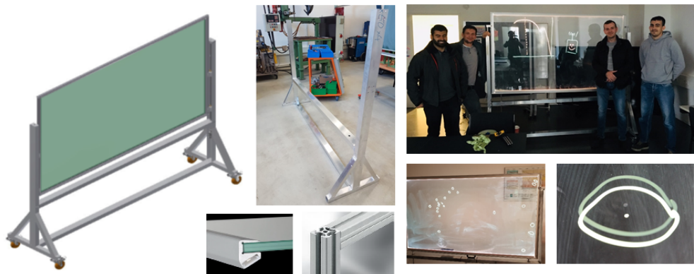
Figure 2. Images of lightboard production and glass micro flaws/precipitations.
