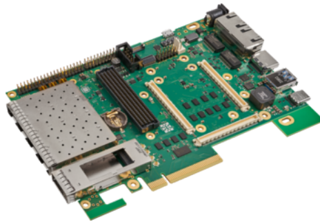
Figure 2.2.3: Picture of a SOM base board. This board includes for example FMC slot, USB and a SFP cages together with a PCIe interface to insert on a computer for versatility.
