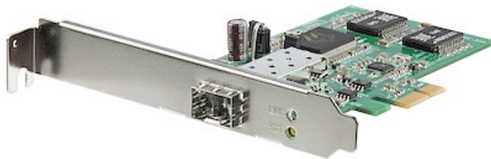
Figure 3.5.1: Startech PEX1000SFP with the RTL8168B chip
