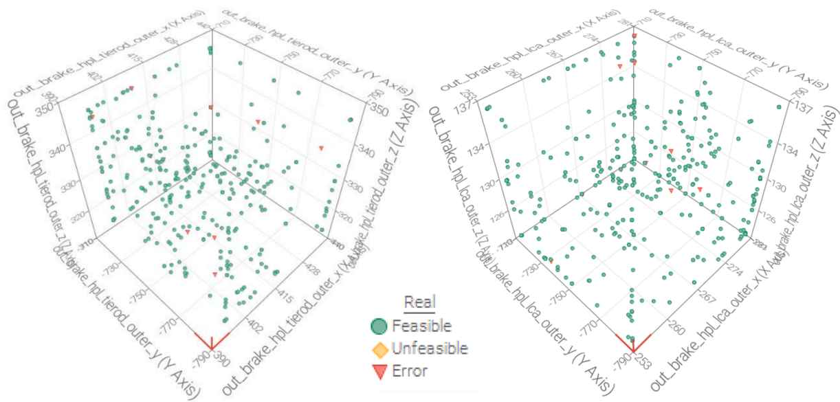
Fig. 5. Scatter plot of the parameter values used in the optimization process regarding the outer hardpoint locations of the left lower control arm and the tierod, in which the dimensions are expressed in mm.
