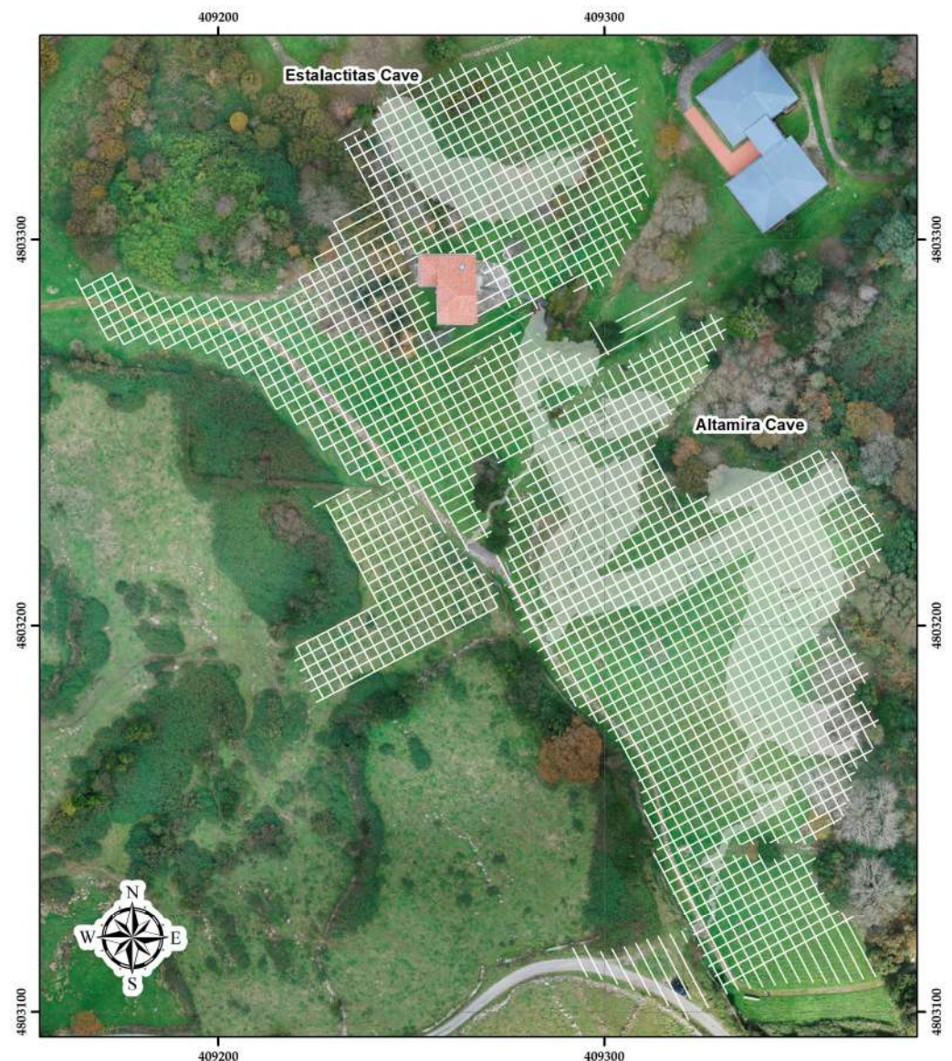
Figure 5. The location of GPR profile grid (orthogonal 2D profiles spaced every 3 m) in the Altamira Cave site, carried out with the 100 MHz antenna.
