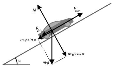
Figure 5. Visualization of road gradient and friction on a car.
