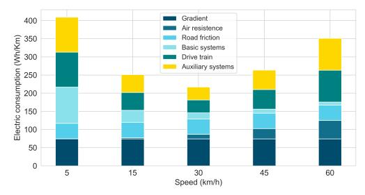
**Figure 6.** Electric consumption categorized by gradient, air resistance, road friction, basic systems, drive train, and auxiliary systems.
