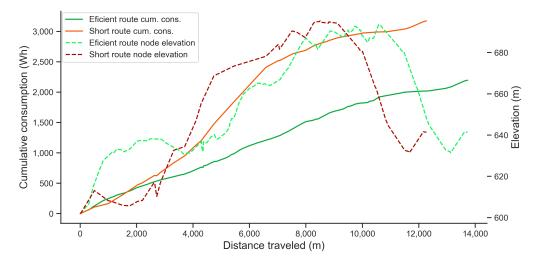
**Figure 9.** Example of a comparative analysis of electricity consumption and elevation during a vehicle trip. The dashed lines represent how the elevation changes along the distance. The solid line represents the cumulative consumption values.
