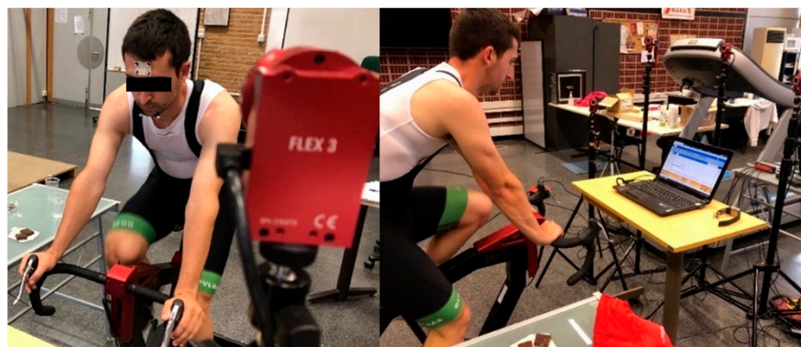
Figure 2. Cyclist with markers placed on his jaw and forehead during the test.
