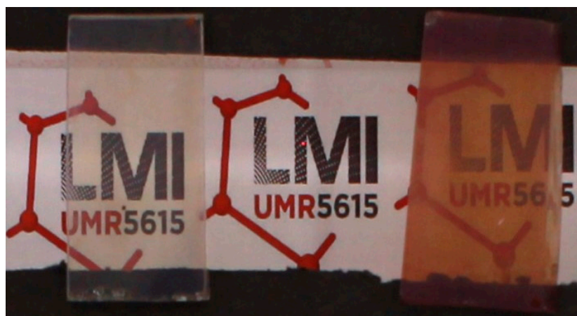
Figure 5. Photographs of MOF thin films in a controlled light environment for Al-PMOF from 200 cycles alumina ALD film (left) and Zn-Al-PMOF from 300 cycles alumina ALD film (right). To demonstrate the good transparency and clarity, the films were lifted 3 cm away from the surface.
