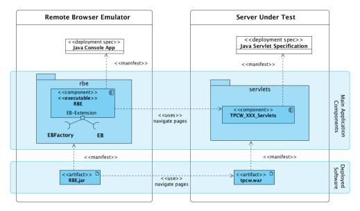
Figure 5.2: Main software components of TPC-W Java implementation
