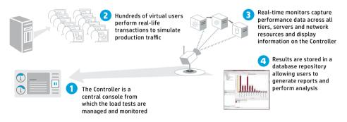
Figure 2.10: How LoadRunner works
