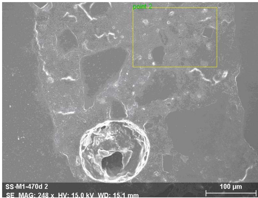
(B) A point falls at distance 2.052mm from the sample surface after 470 days of degradation
