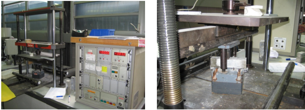
Figure 3-7 Procedure of flexural test
