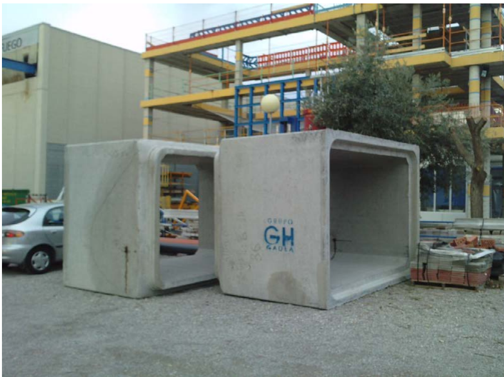
Figure 3-2 Precast concrete frames on AIDICO facilities.
