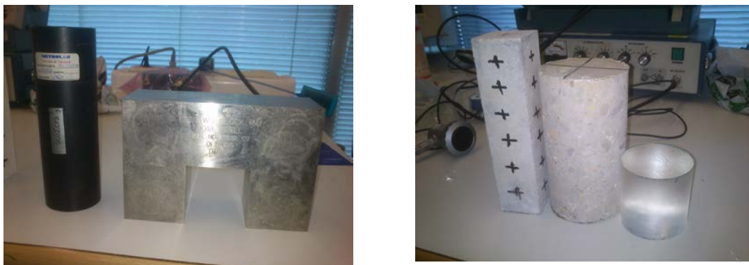
Figure 3-9 Reference blocks used for the equipment calibration
