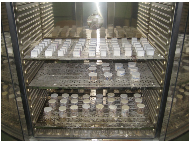
Figure 3-8 Procedure of porosity measurement
