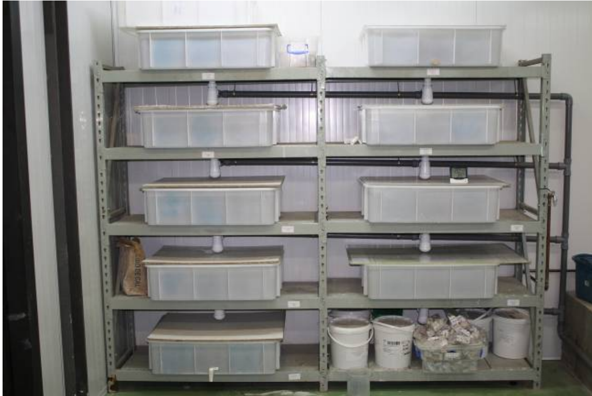
Figure 3-5. Some of the plastic boxes used in the entire research with 120 x 80 x 25 cm. of dimensions, in the durability chamber at AIDICO.
