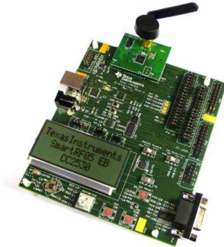
Figura 3.4: SmartRF05 Evaluation Board con CC2530EM
