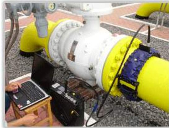
Figure 2 WaveMaker G3, Guided Ultrasonics, Ltd
