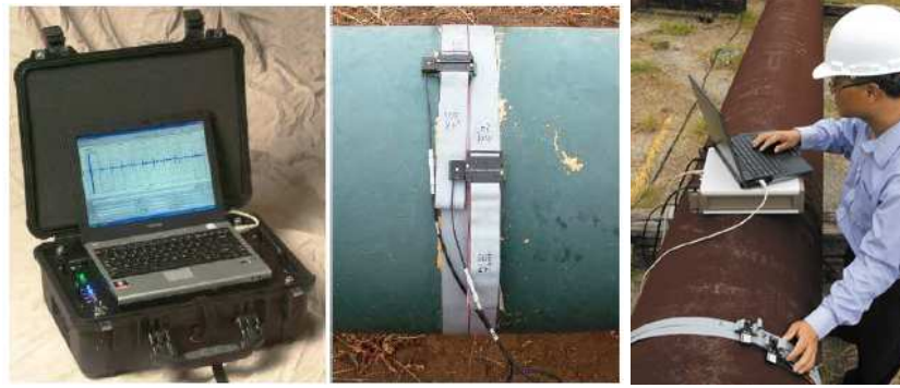
Figure 27: MsSR3030R system (source: Guided Wave Analysis LLC, 2012)
