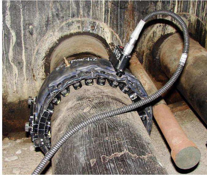
Figure 4. A piezoelectric guided wave piping probe (source: Guided Ultrasonics Ltd., 2009)
