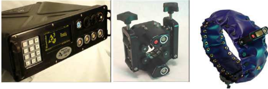
Figure 25. Wavemaker G3 system (source: Guided Ultrasonics Ltd, 2012)
