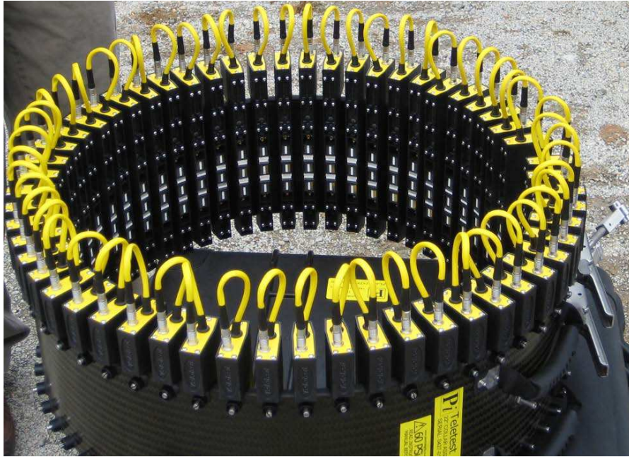
Figure 6. Teletest probe containing well over 100 transducers (source: TWI ltd, 2009)
