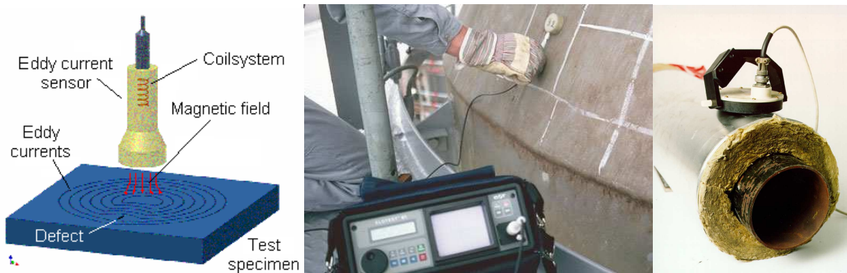
Figure 37. Eddy current inspection method (source: GE NDT, 2011)
