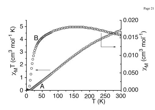
Figure 4. Plots of  $\chi_M T$  versus T (A) and  $\chi_M$  versus T (B) for 1 from 2 to 300 K in 0.08 T field.
