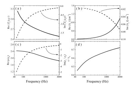
FIG. 3: Real and imaginary parts of: (a) characteristic impedance  $Z_c$ ; (b) propagating wave vector  $k_c$ ; (c) dynamical mass density  $\rho$ ; and (d) effective sound speed c. Note that parameters are determined from density  $\rho$  and bulk modulus K, which are the two independent parameters in the model (see text).
