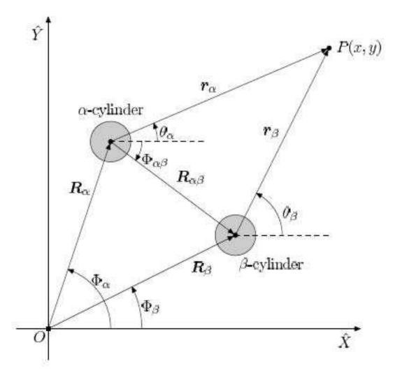
FIG. 1: Coordinate system and variables used in the multiple scattering theory.
