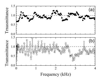
FIG. 7: (a) Transmittance of a flat perforated metal plate 0.5 mm thick. The perforations are circular with 0.5mm diameter and are arranged in a hexagonal lattice.(b) Transmittance through a SC structure consisting of three rows of cylinders (8 cm diameter) fabricated with the perforated plates characterized above. The dashed horizontal lines are guides for the eye.
