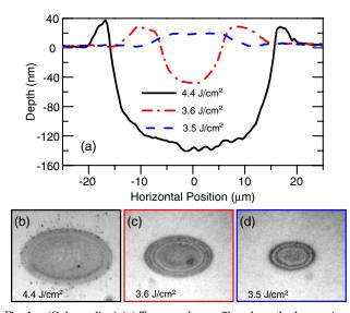
Fig. 1. (Color online) (a) Topography profiles along the long axis of single pulse irradiated regions in phosphate glass at three different laser fluences (see labels). (b)–(d) Optical micrographs of the laser-exposed regions shown in (a). The field of view is in all cases  $46 \times 39 \ \mu m^2$ .
