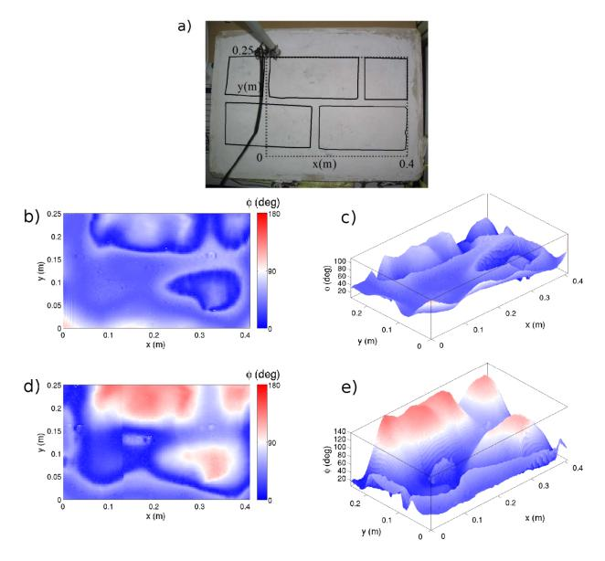
In addition, we tested another sensor configuration in terms of their orientation. The emission was perpendicular to the test specimen surface and two symmetrical receivers forming an angle to the test specimen were used. However, the results obtained with this configuration did not provide clear information about the position where the bricks are located.
