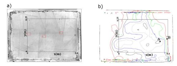
The maximum change in height variations occurs for distances greater than 6 cm. Figure 7(b) shows that the maximum height gradient exists between points A and B. In the results shown in Figure 6, there are angular delays greater than 73.33° between points located very close to each other. On the other hand, observing the contour lines in Figure 7(b), there is no correspondence with the geometry and brick arrangement of the test specimen.
