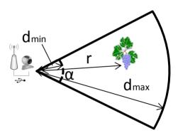
The field of view (FoV) of a camera (if the image system is rectilinear) depends on the collimator focal length and the target size (assuming the sensed image includes the whole target). It can be estimated by Equation (5):
