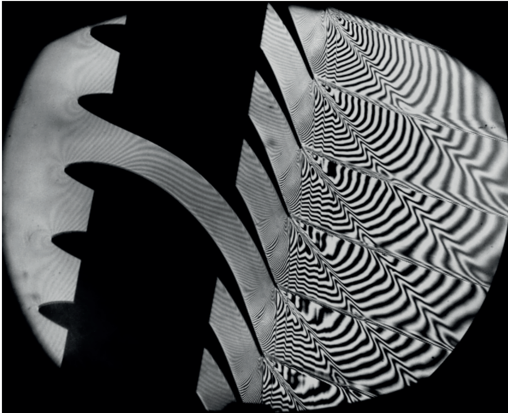
Fig. 1: Interferogram taken at isentropic exit Mach number M_{2is} = 1.828 and angle of incidence i = 0^\circ
