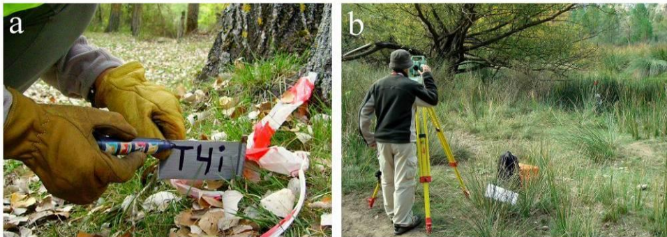
Figure 3.7. Example of a steel rod marking out the location of one cross-section (a) and geo-referenced survey of vegetation units in CRA using a total station (b).
