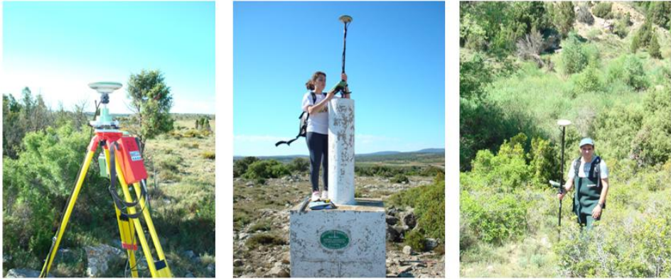
Figure 2.4. Assignment of absolute coordinates to the site Mijares-Terde with GPS. Base station (left) and rover in the Molino geodesic point (centre) and in the study reach (right).
