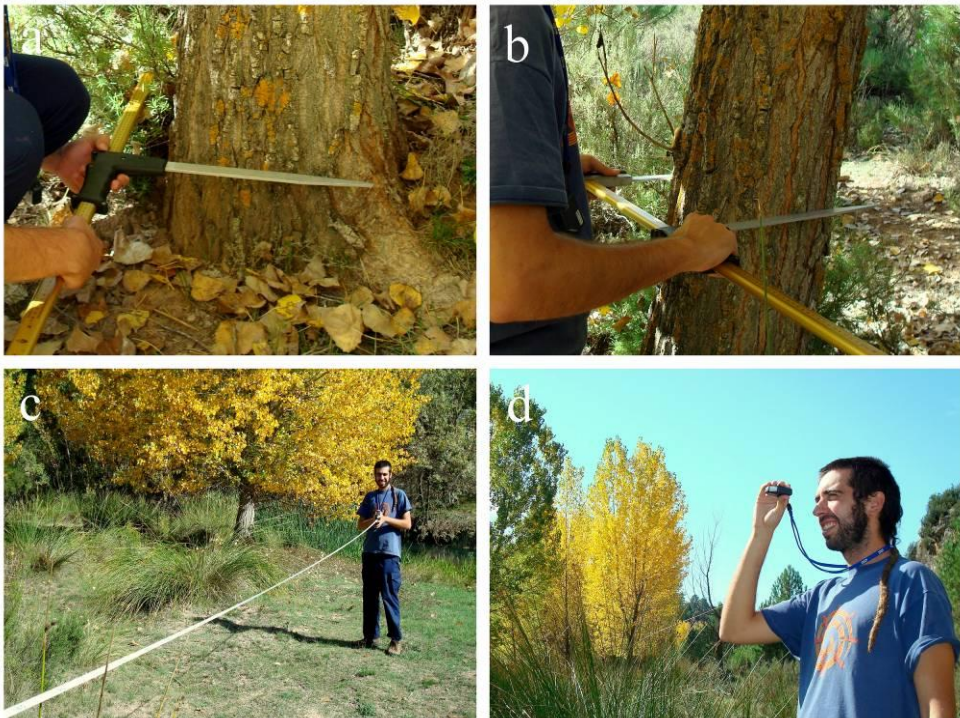
Figure 3.10. Measurement of the diameter at ground level (a) and diameter at breast height (b) using a caliper, and measurement of the height of a tree, using a measuring tape to set the distance (c) and an electronic clinometer (d).
