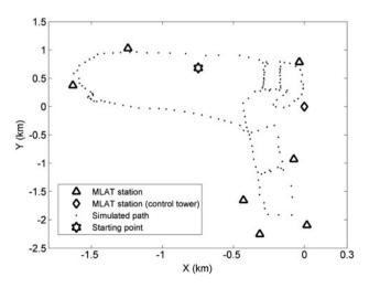
Fig. 2. Linate airport system layout.
