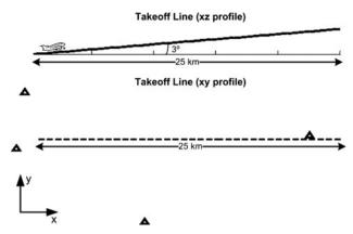
Fig. 6. Layout of the MLAT system for a takeoff line.
