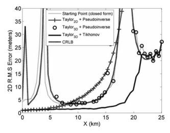
Fig. 7. Horizontal accuracy over the takeoff line.
