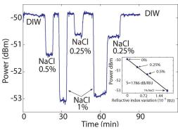
Fig. 5. (Color online) Time evolution of the output power during the flow of NaCl dilutions with different concentrations. The inset shows the sensitivity curve.
