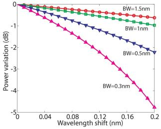
Fig. 2. (Color online) Power variation versus wavelength shift for different initial alignments between the source and the sensor. BW, initial overlapping bandwidth.
