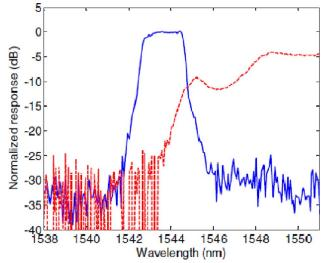
Fig. 4. (Color online) Normalized transmission spectra of the corrugated waveguide (dashed red line) and CFBG-filtered optical source (solid blue line).
