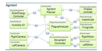
Figure 3: Software architecture of the Agrobot
