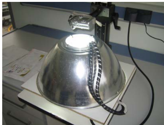
Figure IV-2. Photography set (illumination system, column and digital camera)
