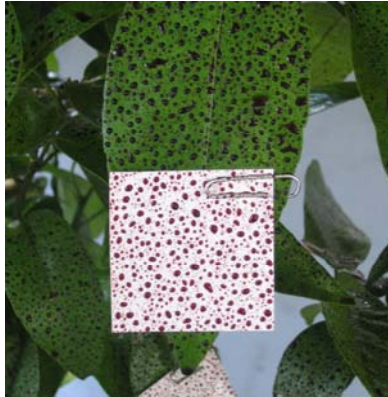
Figure IV-1. Example of spray distribution on a citrus leaf and a PVC collector.
