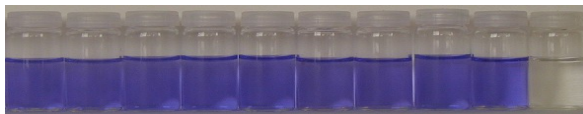
Figure 1 Colour changes observed for acetonitrile solutions of chromoreactand 1 ( 1.0 \times 10^{-4} mol dm -3 ) in the presence of 10 equivalents of the correspondent anion (except for cyanide; 1 equivalent). From left to right: no anion, Cl - , Br - , I - , NO 3 - , AcO - , H 2 PO 4 - , HSO 4 - , NCS - and CN - .
