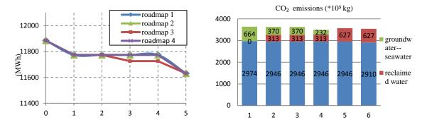
**Figure 4.4.** Energy required for pumping in baseline scenario (1) and throughout the steps of roadmap 1 (2-6) (left panel) and for potable water treatment (right panel).
