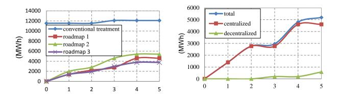
Figure 4.5. Energy required per month for the conventional and advanced treatment of wastewater (left panel) and energy required for the advanced treatment of wastewater throughout the five steps of roadmap 3 (right panel).
