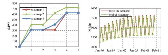
**Figure 4.3.** Monthly timeseries of energy consumed for pumping water from water resources (left panel) and energy required for pumping treated wastewater (right panel).
