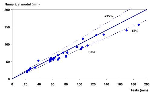
Fig. 5. Comparison of fire resistances between the numerical model and tests.
