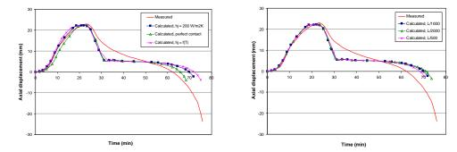
Fig. 7. Comparison of measured and predicted axial displacement with different gap conductance values.
