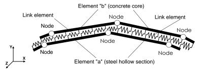
Fig. 1. Specific composite bar element.
