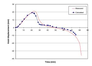
Fig. 3. Comparison of measured and predicted axial displacement, column C-17.
