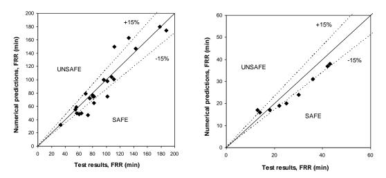
Fig. 4. Comparison of FRR between the numerical predictions and the test results (Canadian tests).
