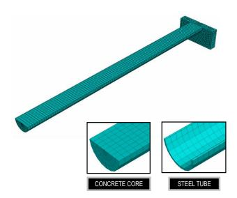
Fig. 1. Finite element mesh of the model.
