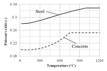
Fig. 4. Temperature-dependent Poisson's ratio.
