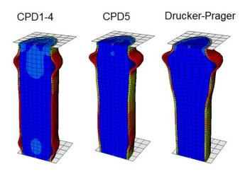
Fig. 6. Comparison of deformation shapes for different concrete models.
