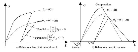
Fig. 2. Procedure to change from a stess-strain curve to another.
