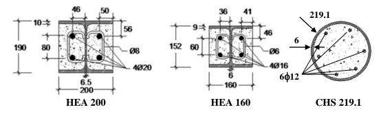
Fig. 2. Scheme of the cross-sections of the studied columns (dimensions in mm).
