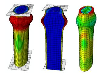
Fig. 3. Deformation of FE model.
