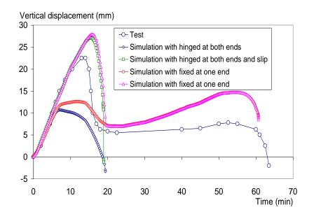
Fig. 3. Vertical displacement at the column top.
