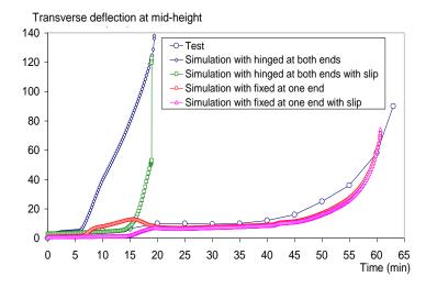
Fig. 4. Transverse deflection at mid-height of column.
