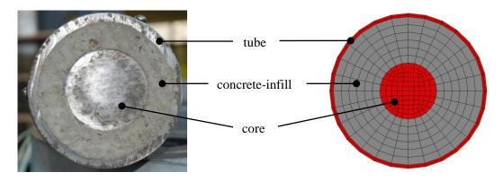
Fig. 1. Cross-section of concrete-filled column with embedded steel core.
