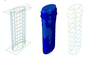
Fig. 8 Deformation of concrete and reinforcement.
