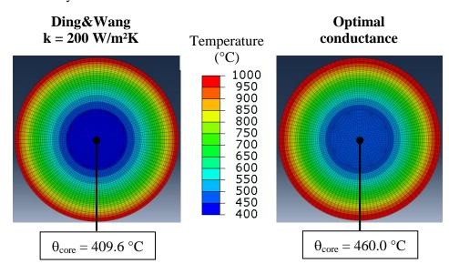
Fig. 5. Temperature distribution through cross-section for different thermal contact properties.
