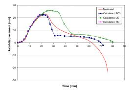
Fig. 9. Comparison of measured and predicted axial displacement with different steel models.
