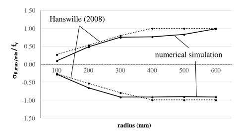
Fig. 6. Maximum and minimum residual stresses in massive circular steel sections.
