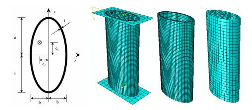
Fig. 2. FE model for selected test specimens
