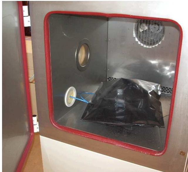
Figure C.3: Thermal cycling chamber. Device under test is placed in a hermetic bag.
