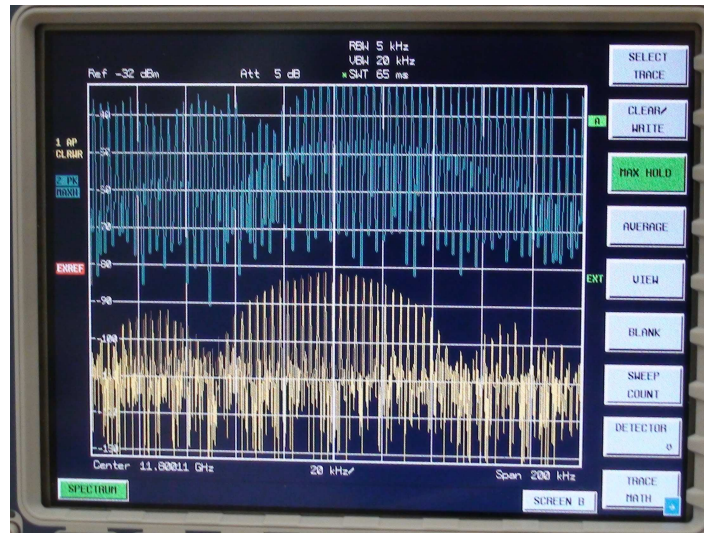
Figure C.10: Screenshot of the spectrum analyser of the nulling detection chain showing a multipactor discharge, indicated by the gap between the maximum curve (blue line) and the lower actual spectrum measurement (yellow line). Note that the attenuators and phase shifters need to be re-adjusted again to null the actual spectrum. The “Max hold” display mode has been activated.
