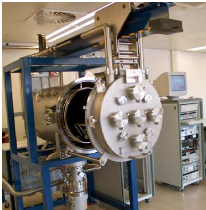
Figure C.1: Vacuum chamber. It reaches a pressure below 10^{-7} mbar.
