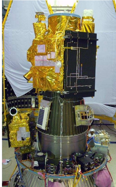
Figure 1.11: Satellite assembly undergoing qualification tests. Multipactor tests are usually conducted for individual payload devices. They are a small, but critical fraction of all required system and subsystem tests. Source: ESA.
