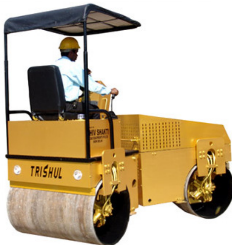
(P21: Vibratory compactor)
