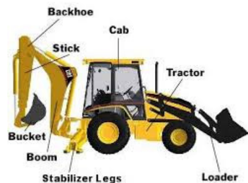
(P19: Excavator with its several parts)
