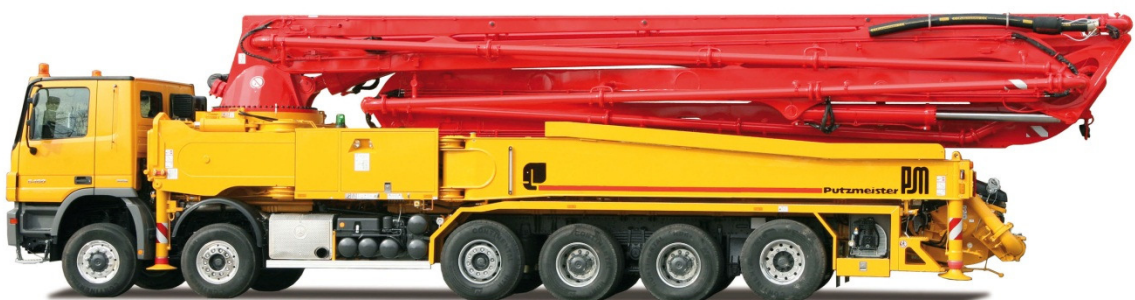
(P30: Concrete pump)
