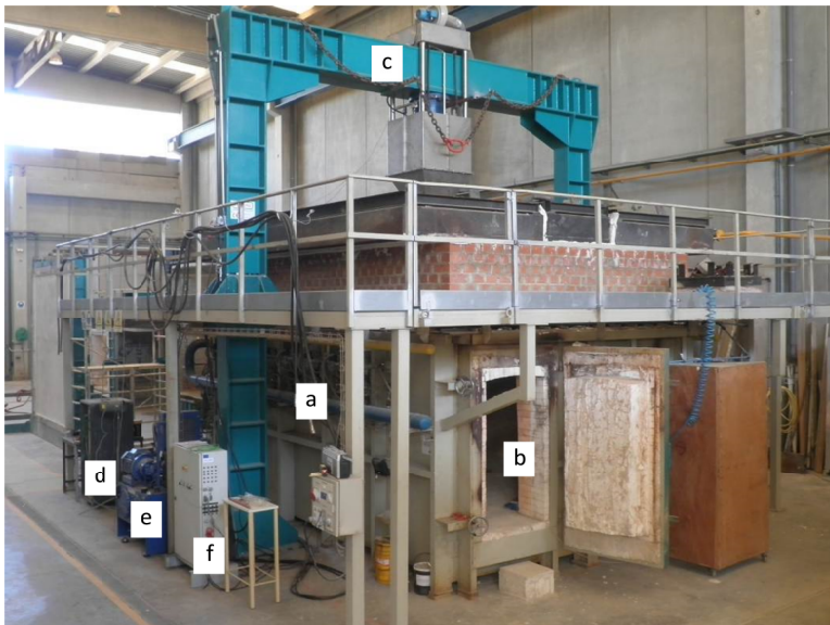
Fig. 2. General view of the testing facilities: a) test furnace; b) furnace access gate; c) loading frame; d) temperature data acquisition system; e) hydraulic loading system; f) load data acquisition system.
