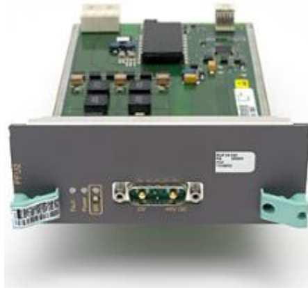
Figura 3.6: Power Filter Unit 2 (PFU2).
