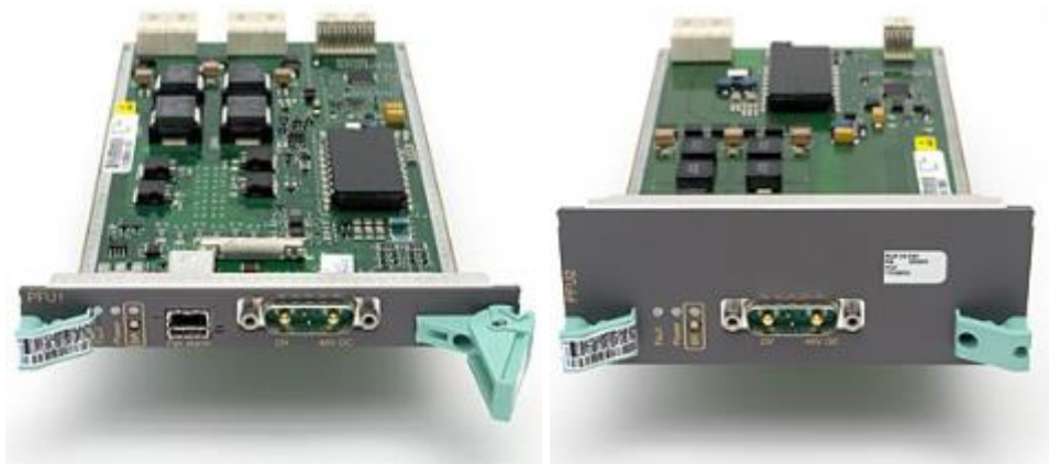
Figura 3.12: Power Filter Unit (PFU).
