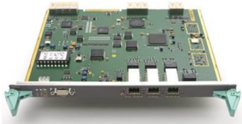
Figura 3.14: Switch Multiplexer Unit (SMU2).
