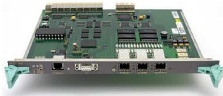
Figura 3.11: Node Processor Unit for AMM 6P/AMM 20P (NPU 8x2).
