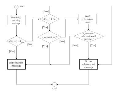
Figure 3: eSBR algorithm flow chart.
