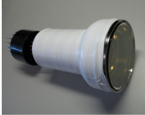
Figure 13. The Hamamatsu R11410-10, a 3-inches photomultiplier with high quantum efficiency ( > 30\% ) at the xenon scintillation wavelengths and low radioactivity.
