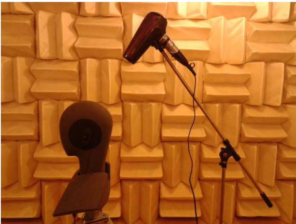
Fig. 2.1. Recording of hairdryer 2 with artificial head recorder in semi-anechoic chamber in Technische Universität Berlin.
