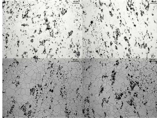
Figure 5.7: Pellets type T microsections showing the fine porosity as well as the some pore clusters.
