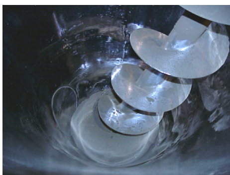
Figure 3.7: Conical screw hopper blender with orbital screw blender.
