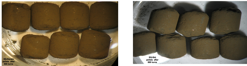
Figure 5.33: Keratin fiber and standard pellets after 600 turn testing.
