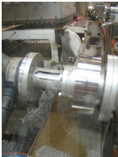
Figure 4.6: Picture showing green pellets chips produced during pressing.
