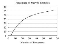
Figure 1: Absolute number and percentage of requests suffering starvation due to protocol races according to the system size. These values are the average ones for all applications cited in Section 6 (Table 2)
