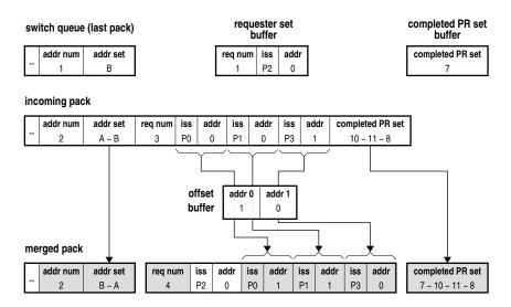
Figure 8: Packing example. Iss refers to issuer, addr to address location, and req num to request number
