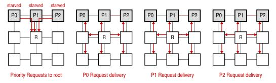
Figure 2: Routing of priority requests through ordered paths. R is the root switch of the ordered path by several responses on just one. Thus, instead of having to wait for a response from each sharer, only few responses will be received. This will reduce the write latency and will alleviate the congestion of the buffers, mainly in the writers.
