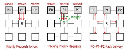
Figure 3: Packing several priority requests into just one on coinciding at switch R
