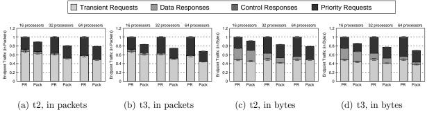
Figure 11: Normalized total endpoint traffic. PR stands for Token Coherence using only normal priority requests and Pack stands for Token Coherence using the packing technique
