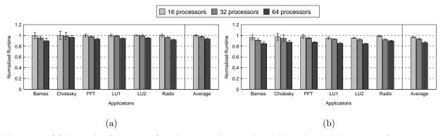
Figure 18: (a) Normalized runtime of applications when applying the packing technique to token responses and (b) normalized runtime when applying packing simultaneously over priority requests and token responses
