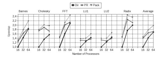
Figure 19: Speedup of applications in a 16, 32, and 64-processor system when using a directory-based protocol (Dir), TokenB using priority requests (PR), and TokenB using priority requests and the packing technique over priority requests and token responses with suitable timeout (Pack). Data are normalized to those for the directory protocol in a 16-processor system
