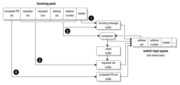
Figure 7: Use of the auxiliary buffers in the packing process
