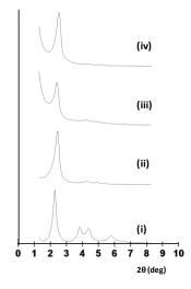
Fig. 1 XRD Patterns for the nanoparticulated MCM-41 as-synthesized (i), calcined MCM-41 nanoparticles (ii), S1 (iii) and S1-CPT (iv).
