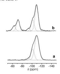
$_{55}$  Fig.5  $^{29}$  Si-NMR of the MCM-41 as synthesized (a) and S1 (b) showing the evolution of the  $Q^2{+}Q^3 and\ T$  sites through the loading and functionalization process.
