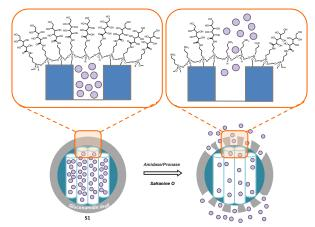
**Scheme 1** Schematic representation of the synthesis procedure and the <sup>85</sup> gate-opening mechanism of **S1** in the presence of the appropriate enzyme.
