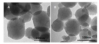
**Fig. 2** Representative Transmission Electron Microscopy (TEM) image of the calcined MCM-41 nanoparticles (A) and the loaded and functionalized mesoporous silica nanoparticles (**S1**) (B).
