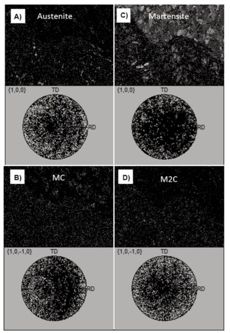
Figure 5. Pole figures of the present phases before tempering.
