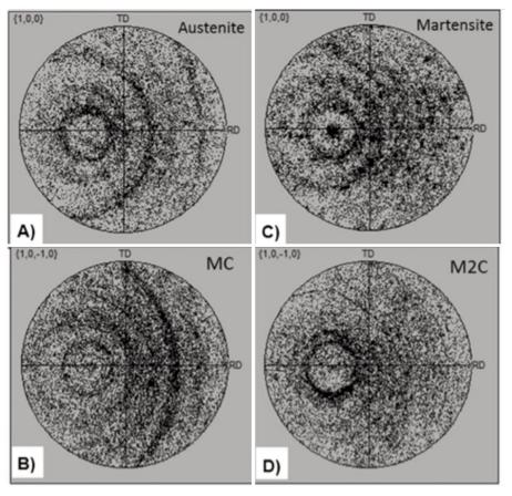
Figure 6. Pole figures of the present phases after tempering.
