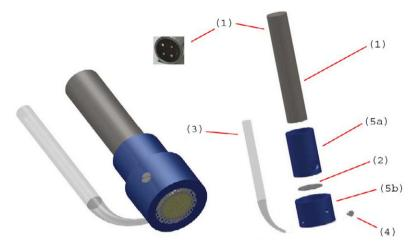
Fig. 1. Wet E-Nose sketch: (1) Electronic Nose; (2) membrane; (3) reference electrode and LPDE adapter; (4) nylon screw; (5) PVC adapters
