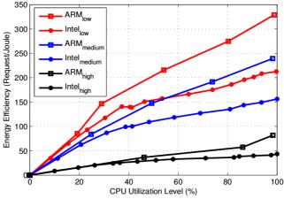
Figure 1-1: Energy-efficiency vs. CPU Utilization Level [Ou 2012]
