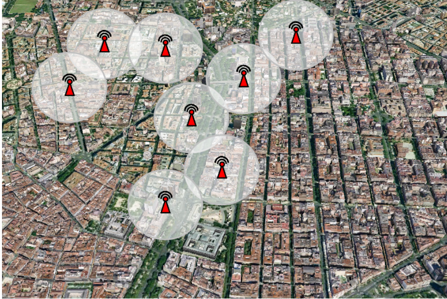
Figure 4.2: Example of 8 RSUs deployed following the Minimum Cost deployment policy.
