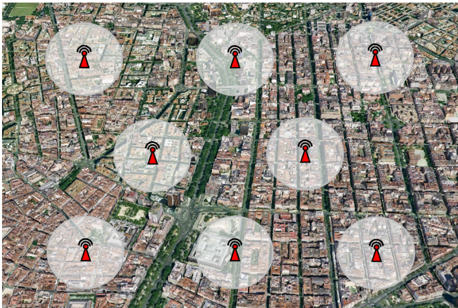
Figure 4.3: Example of 8 RSUs deployed following the Uniform Mesh deployment policy.
