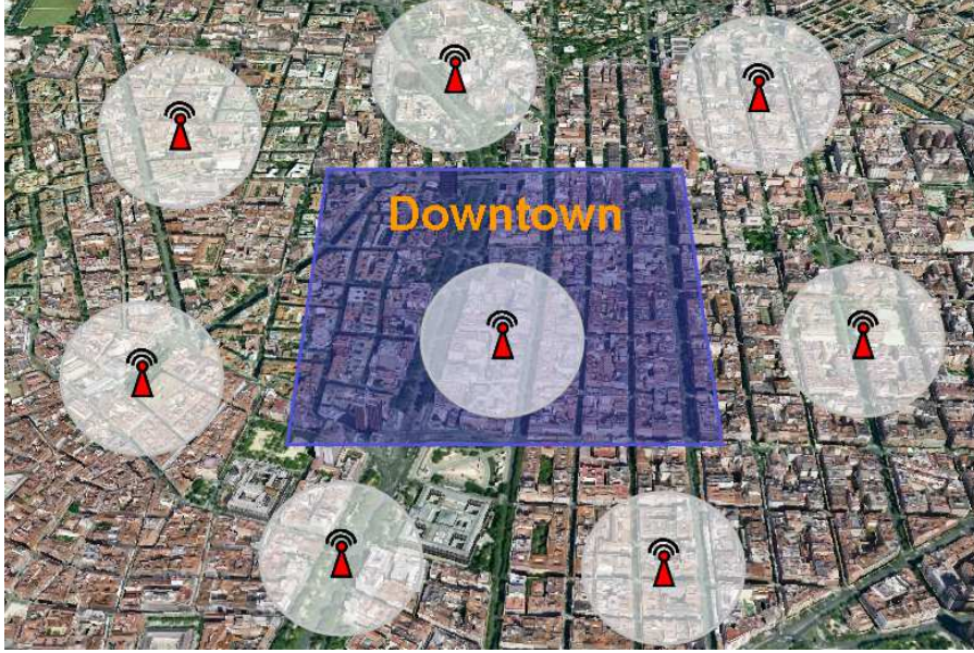
Figure 4.1: Example of 8 RSUs deployed following the D-RSU deployment policy.
