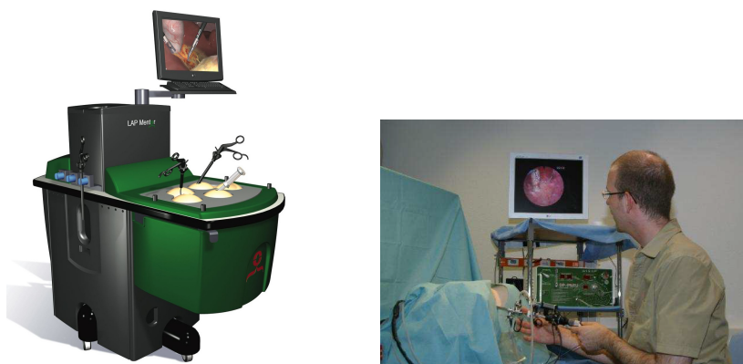
Figure 1.1: The LAP Mentor Virtual Reality laparoscopy simulator from [Ayodeji et al., 2007] (left) and the immersive training environment for hysteroscopy from [Harders et al., 2003] (right).
