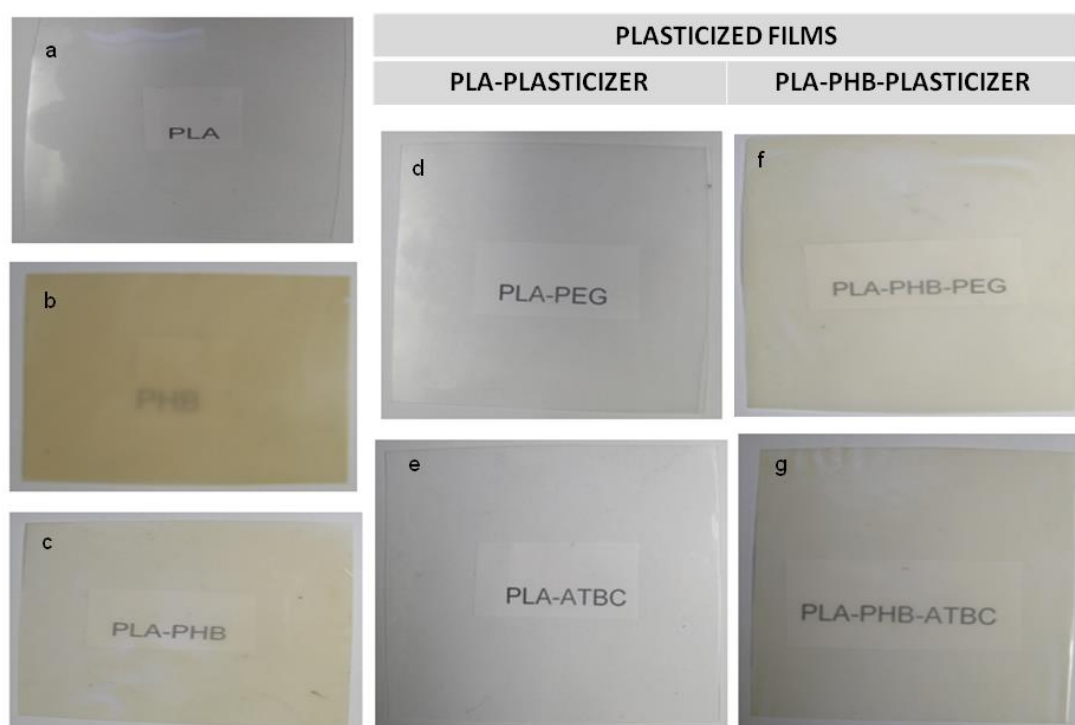
Figure III.4.1. Visual appearance of: a) PLA, b) PLA-PEG, c) PLA-ATBC, d) PHB, e) PLA-PHB, f) PLA-PHB-PEG and g) PLA-PHB-ATBC.
