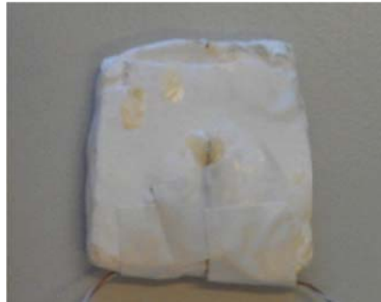
Figure 1. PCM plate obtained from PCL/RT5 fibers.
