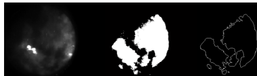
Fig. 3 – Scheme of processing steps. From left to right: original image, binary image of the flame area and binary image of the flame contour
