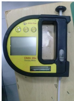
Figura 4.6. Anton Paar DMA in situ
