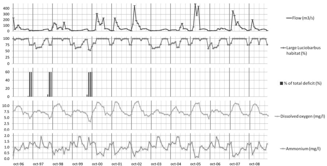
Figure 8. Simulation-Indicators for the scenario with operating rules –OR– at point 4. The river flow is indicated, together with the indicators regarding fish habitat, deficit of supply for irrigation and water quality.
