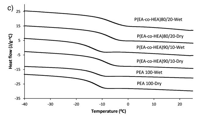
**Figure 1**. DSC heating thermograms of the different copolymer networks. (a) P(EA-co-MAAc) 80/20 and P(EA-co-AAc) 80/20 thermograms in the whole temperature range of the measurements (b) P(EA-co-MAAc) and P(EA-co-AAc) thermograms in the temperature range of the PEA-rich phase transition (c) P(EA-co-HEA) copolymer network thermograms.
