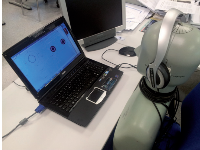
Figure 5.12. Developed headphone-based spatial application running on a notebook with the GPU GTS360M.
