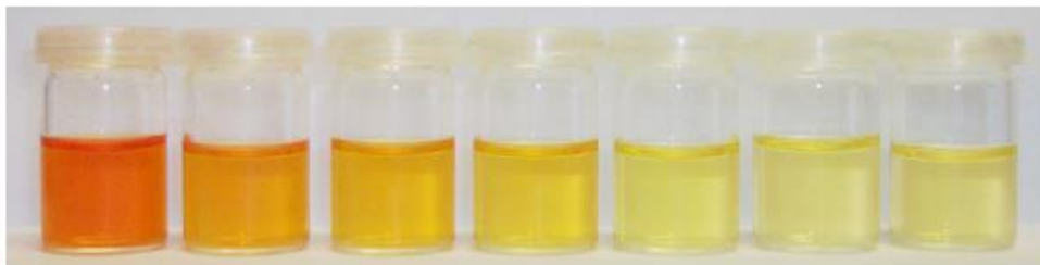
Figure S8. Photograph showing ACN-HEPES (30 mM, pH 7.5) 1:1 v/v solutions of probe 1-Az ( 1.0 \times 10^{-3} M) in the presence of increasing quantities of \text{HS}^- anion. From left to right: no anion, 0.1, 0.5, 0.8, 1.5, 5 and 10 eq. of \text{HS}^- .
