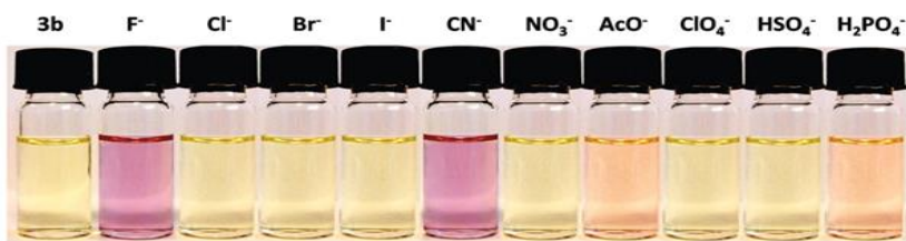
Figure 1. Colour changes of the 3b solution ( 1.2 \times 10^{-4} \text{ mol dm}^{-3} ) seen in the presence of 10 equiv. of \text{F}^- , \text{Cl}^- , \text{Br}^- , \text{I}^- , \text{CN}^- , \text{NO}_3^- , \text{AcO}^- , \text{ClO}_4^- , \text{HSO}_4^- and \text{H}_2\text{PO}_4^- .
